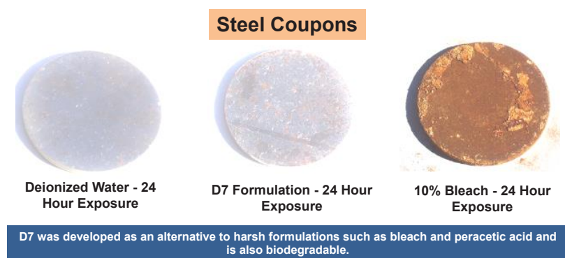
Figure 2: Comparison of the corrosion of D7 vs. 10% chlorine bleach on steel coupons.
